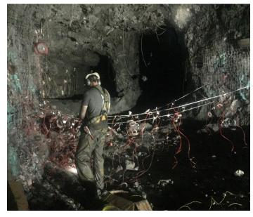
feet in depth. The mine required an electronic detonator with high tensile down-line wire, precise timing, and flexibility both in terms of allowable number of detonators in any one blast and blast duration.
